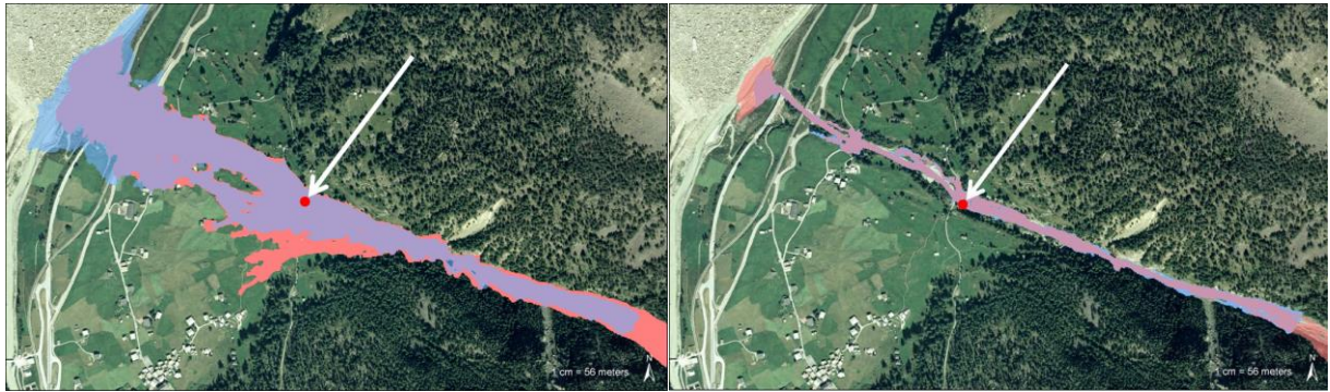
Figure 5.3: Comparison of the inundated areas of a simulation with a vlock release and a hydrograph (a) for a volume of 200'000 \text{ m}^3 and (b) a volume of 2'250 \text{ m}^3 . For all simulations \mu=0.225 and \xi=130 \text{ m/s}^2 . Blue: hydrograph, red: block release. The red points indicate the location of the measured discharge curves (Figure 5.2).
