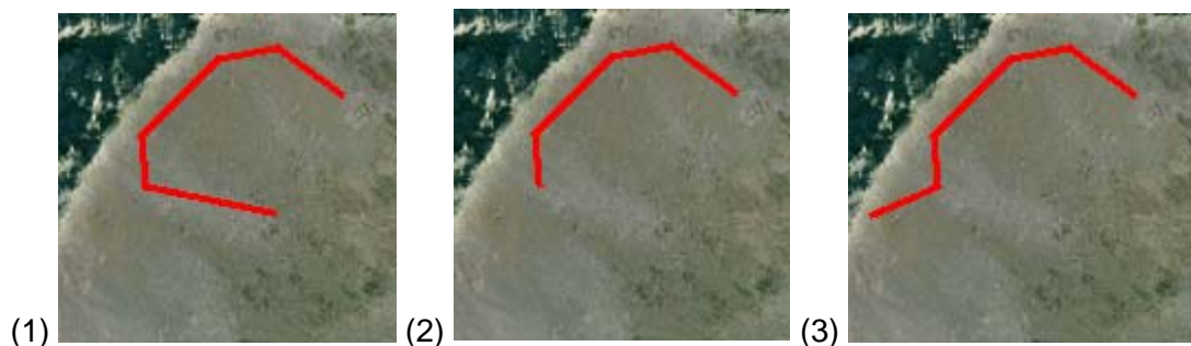
Fig. 1: (1) Draw the release area (in this case counterclockwise), (2) delete the last created point by pressing the mouse wheel and (3) continue drawing the release area.
