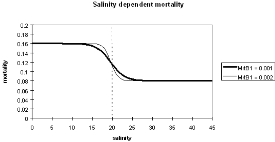
Figure 4.1: Example of the salinity dependent mortality function. m1 = 0.08 \text{ d}^{-1} ; m2 = 0.16 \text{ d}^{-1} ; b2 = 11000 (equivalent with 20 ppt salinity) [\text{gCl m}^{-3}] ; b1 = 0.001 and 0.002 \text{ m}^3 \text{ gCl}^{-1} .
