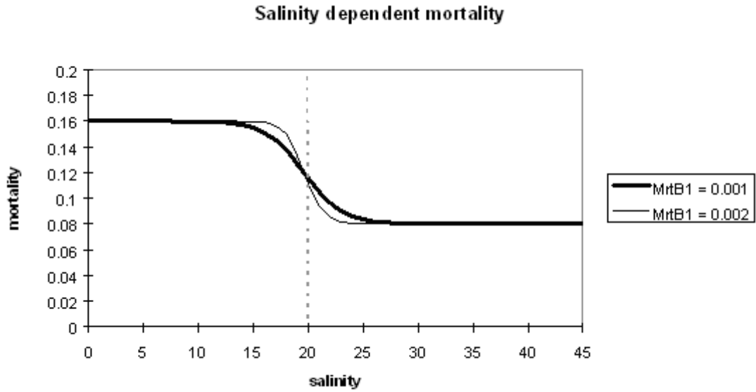
Figure 16.1: Example of the salinity dependent mortality function. m1 = 0.08 \text{ d}^{-1} ; m2 = 0.16 \text{ d}^{-1} ; b2 = 11000 (equivalent with 20 ppt salinity) [\text{gCl m}^{-3}] ; b1 = 0.001 and 0.002 \text{ m}^3 \cdot \text{gCl}^{-1} .
